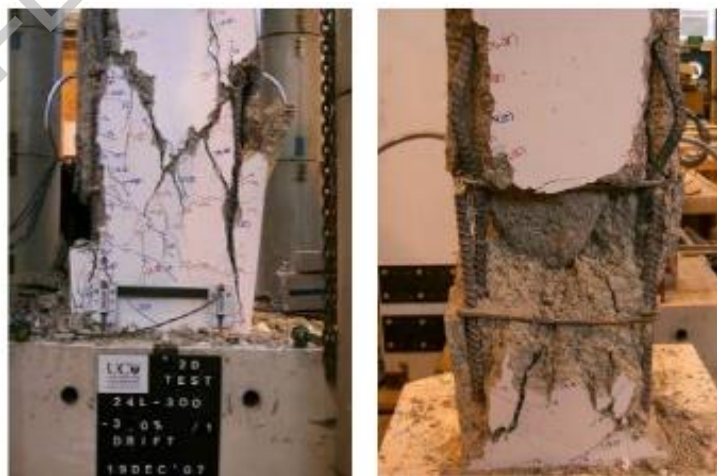
Figure C5.2: Performance of poorly detailed and confined gravity columns designed according to NZS 3101:1982 code provisions (after Boys et al., 2008)
